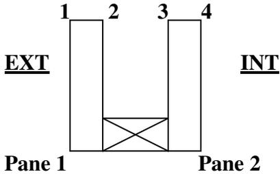
The spacer butts against the glass allowing for heat transfer and also moisture failure.
