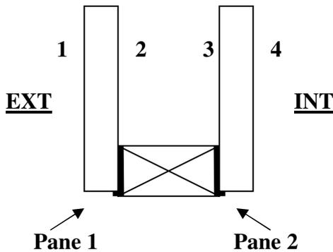
The spacer does not butt against the glass directly but is buffered by a sealant or plastic. This is also known as a double seal. This reduces the energy transfer through the spacers.
